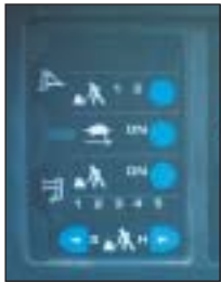
Track shoe slip control panel
