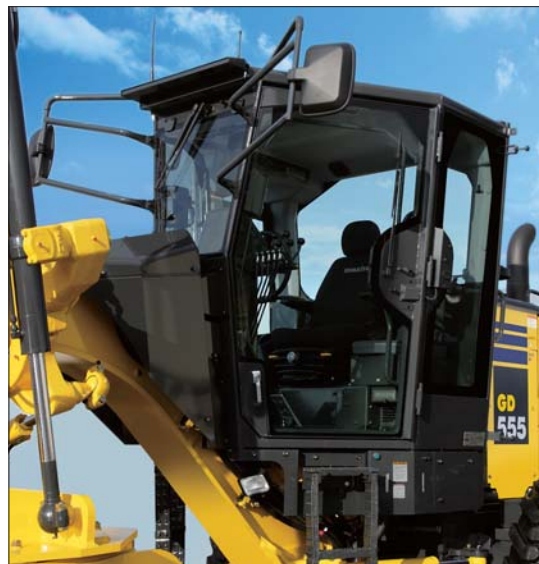
ROPS Cab (Equipped with defroster and intermittent wiper)
