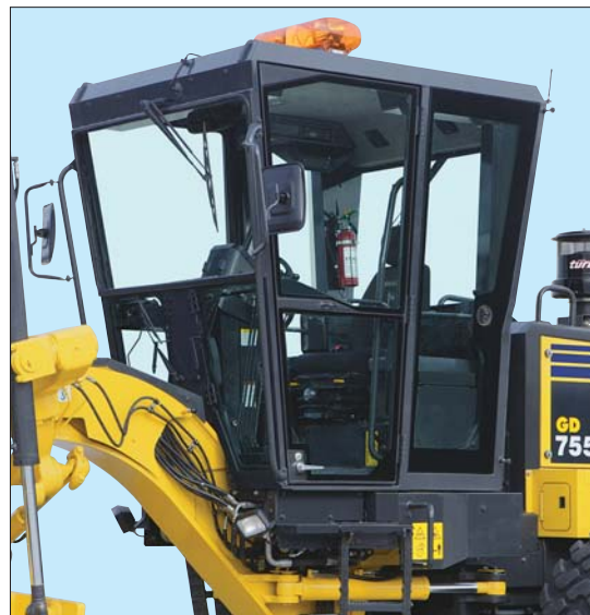
ROPS (ISO 3471) Cab (Equipped with defroster and intermittent wiper)
