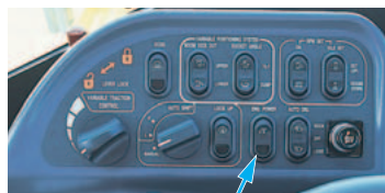
Dual mode engine power selection switch
