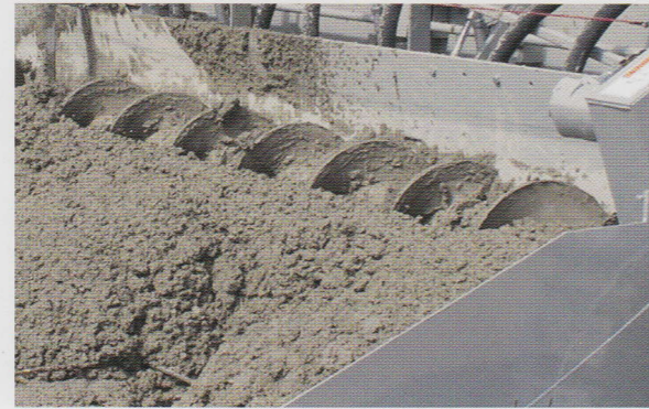
The spread auger and strike-off plate.
